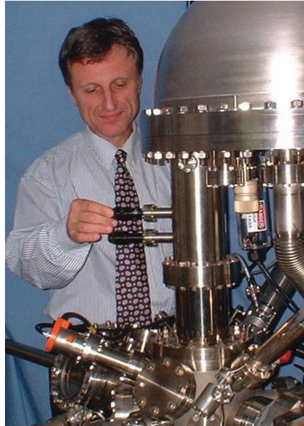
Figure 1 High performance XPS instrument for non-destructive chemical and elemental analysis of materials. The instrument is also capable of high spatial resolution chemical images.
